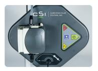
Attempt to restart the OAS pump by pressing the green Start button on the OAS pump control panel and verify that the green LED illuminates.
