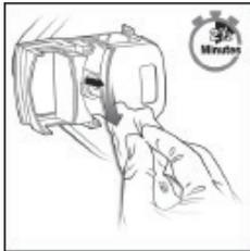
Figure 10. Wipe closure seam
