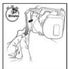
4. Thoroughly wipe the seams and crevices of the pump head cover, around the edges of the lettering, around the button area, and around the power outlet (see Figure 11). Thoroughly wipe all surfaces of the front face of the pump (see Figure 12). Continue to keep all surfaces wet for a minimum of two and a half minutes. Discard the wipes.
