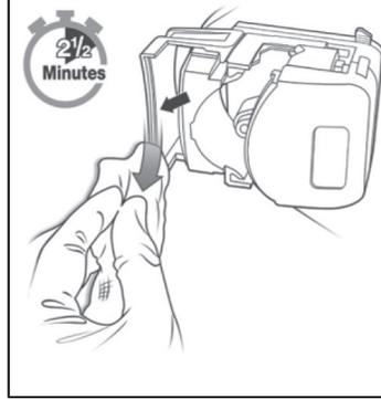
Figure 10. Wipe Closure Seam.
